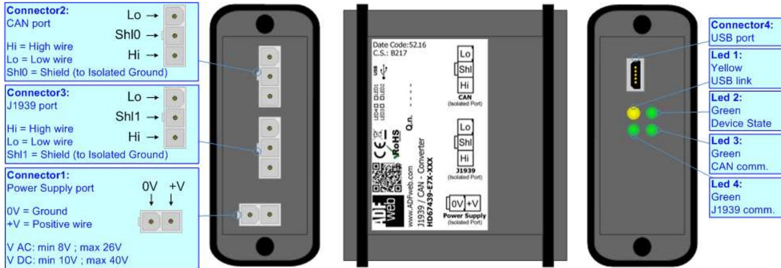
Figure 1a: Connection scheme for HD67439-E4x-xxx
