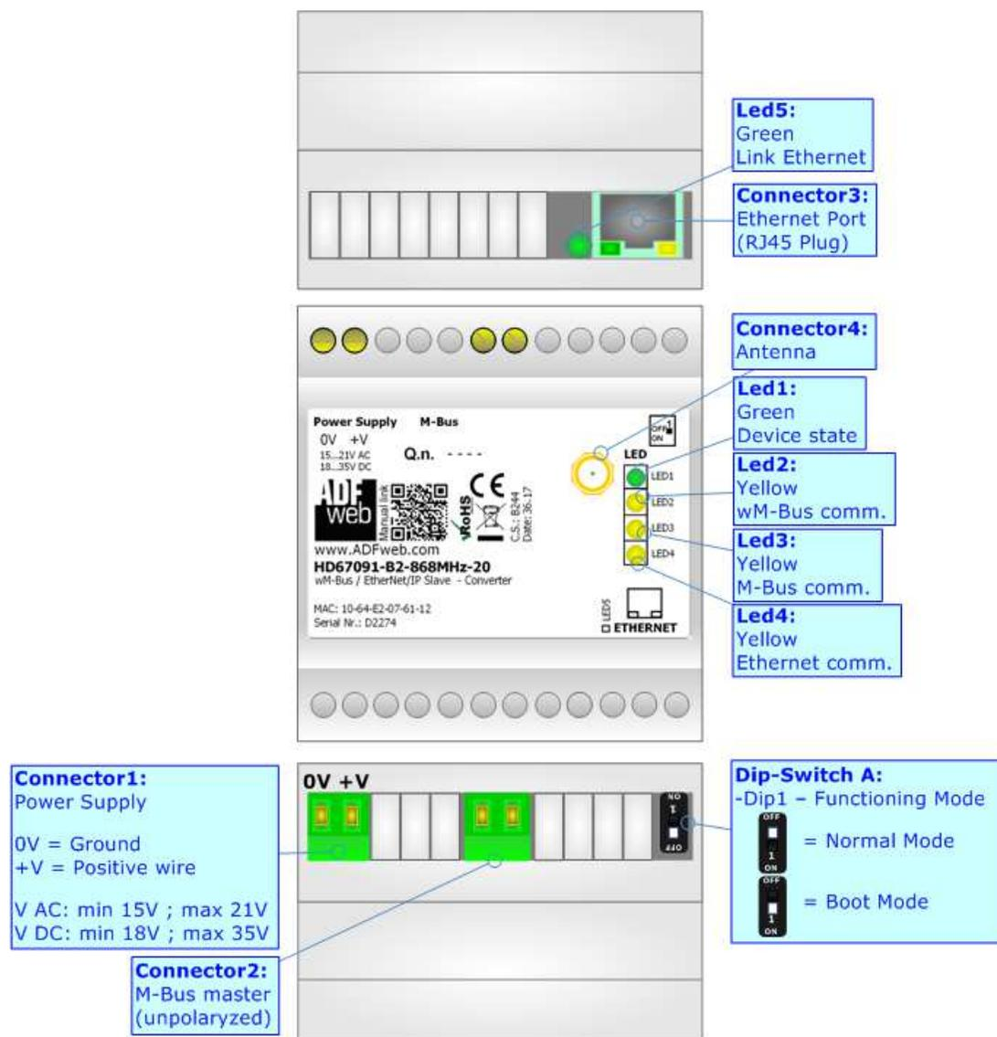
Figure 1b: Connection scheme for HD67091-B2-xxxMHz-xxx
