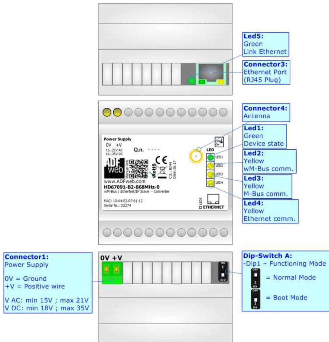
Figure 1a: Connection scheme for HD67091-B2-xxxMHz-0
