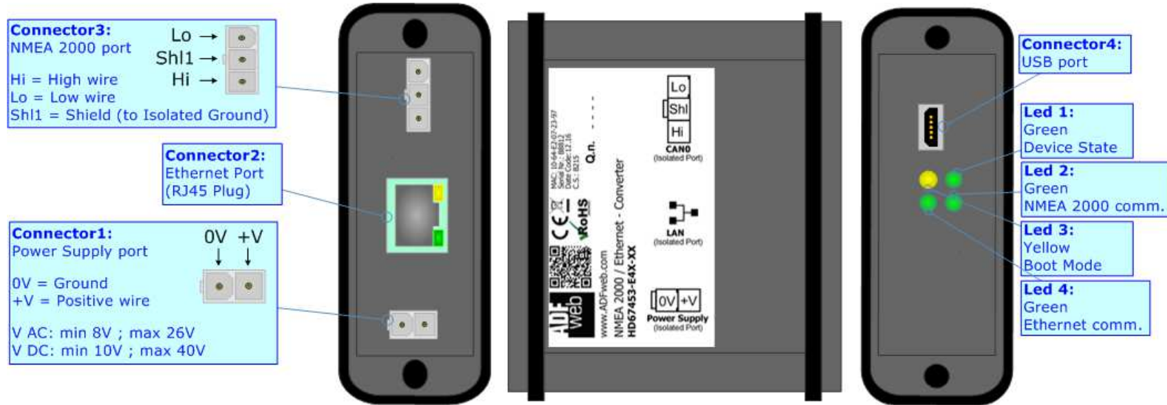
Figure 1a: Connection scheme for HD67453-E4x-xx
