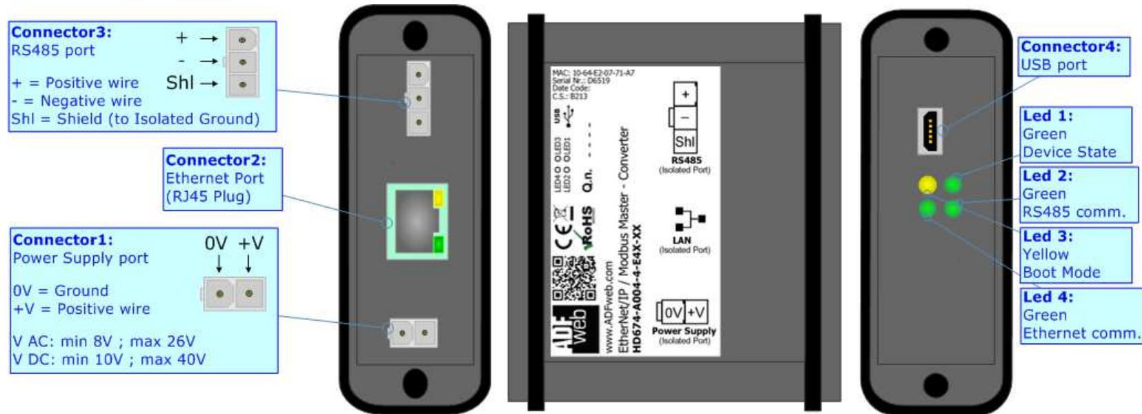
Figure 1c: Connection scheme for HD674-A004-4-E4x-xx
