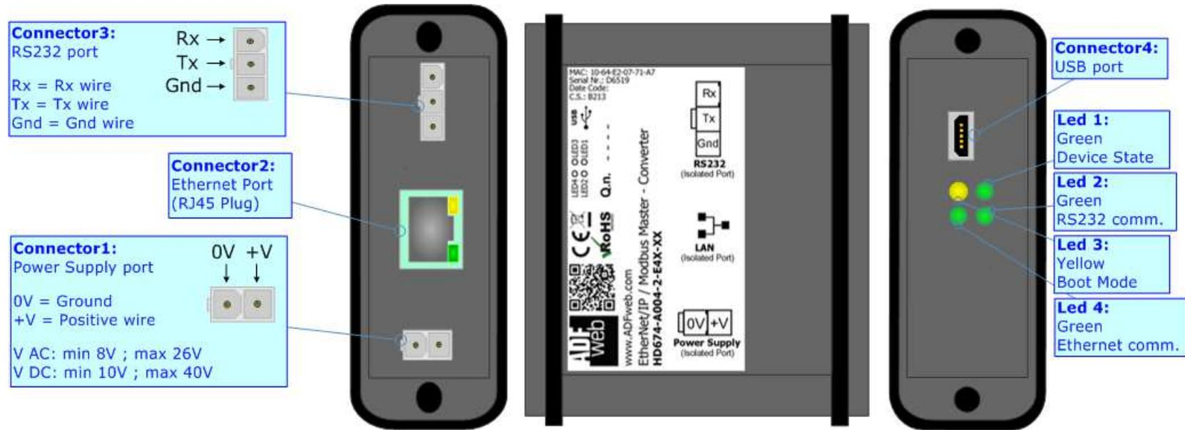
Figure 1a: Connection scheme for HD674-A004-2-E4x-xx
