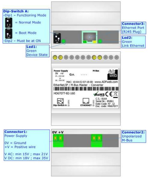
Figure 1: Connection scheme for HD67077-B2-xxx
