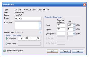
2) Edit the settings of the new Generic Ethernet Module. As shown in the screen shot below, the module was named "HD67077" and the IP-address assigned is 192.168.1.151.
