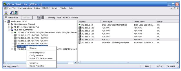
4) With "RSLinks Classic Lite", after have done a network scan (RSWho), and finding the EtherNet/IP device, it is possible to load the EDS file for the device in order to have the "Module Info" compiled.
