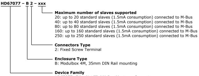
HD67077: EtherNet/IP / M-Bus Master - Converter
