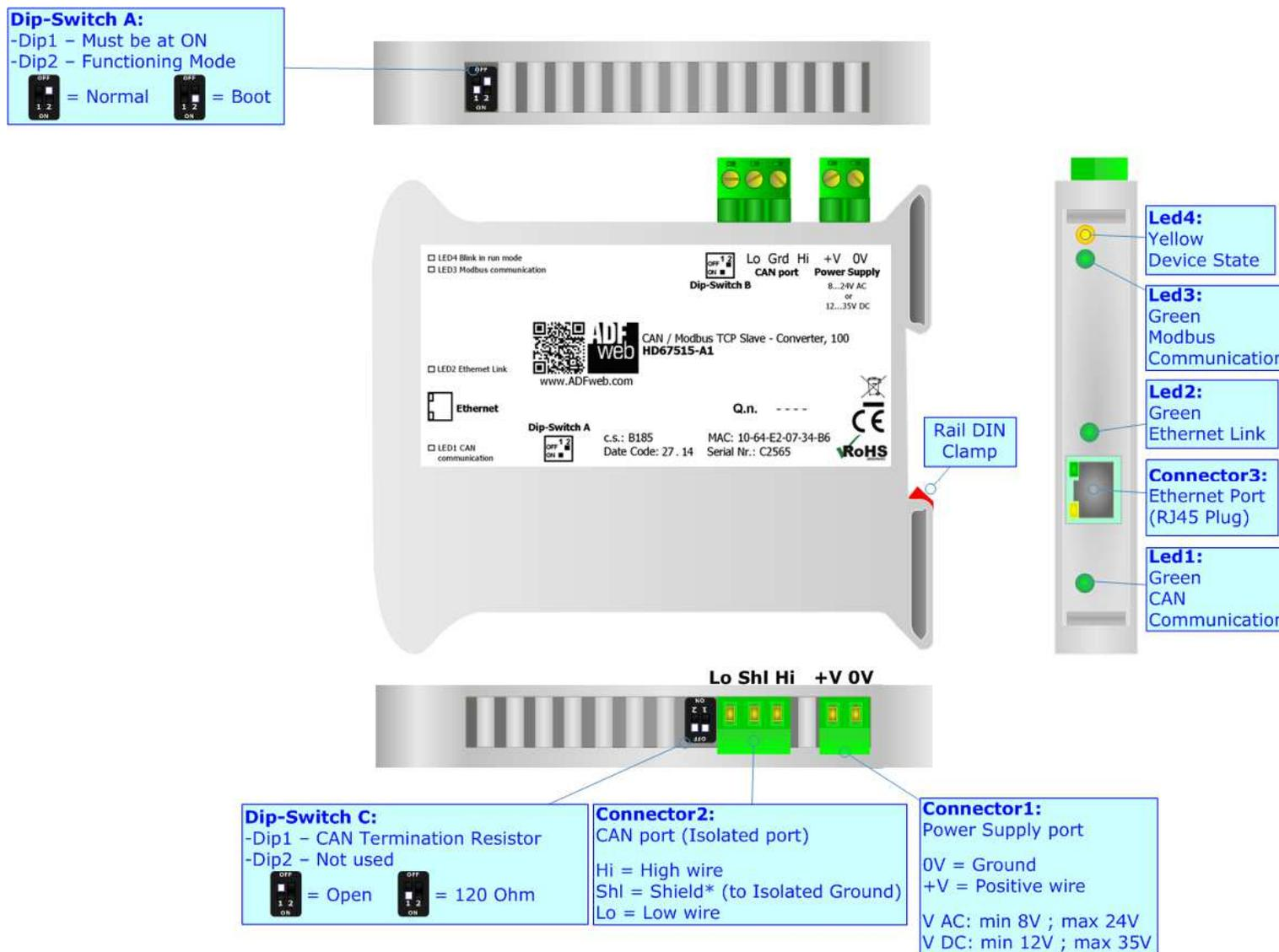
Figure 1a: Connection scheme for HD67515-A1
