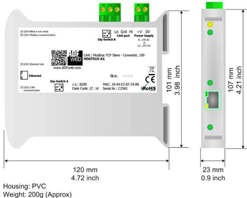
Figure 10: Mechanical dimensions scheme for HD67515-A1
