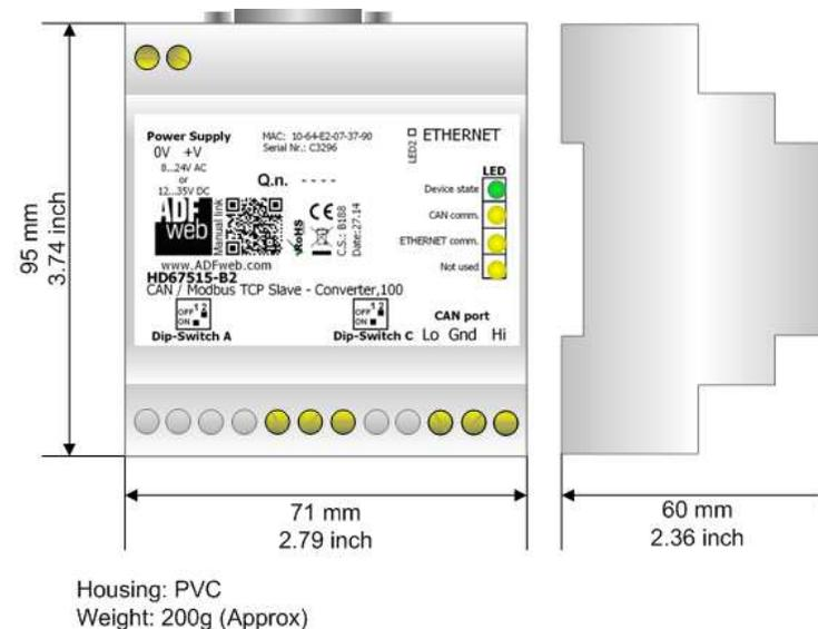
Figure 11: Mechanical dimensions scheme for HD67515-B2
